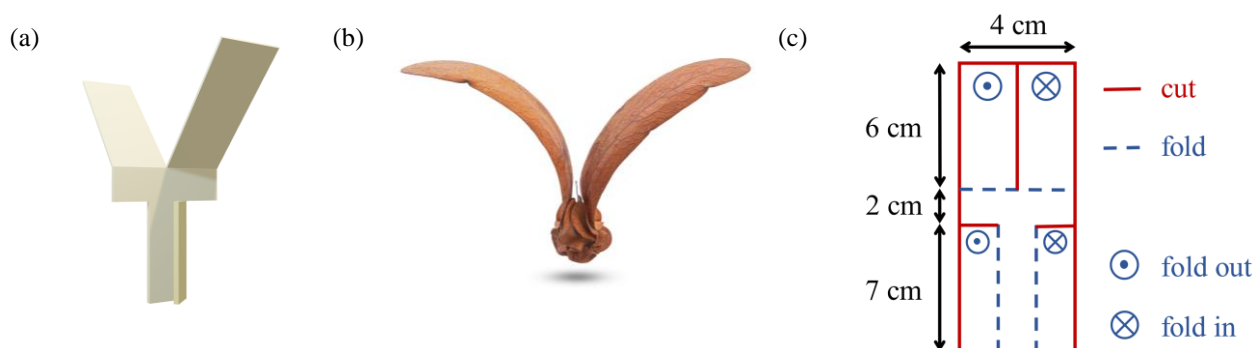
Figure 1. (a) The model of a paper dragonfly. (b) A dipterocarp seed. (c) A demonstration of making a paper dragonfly.
