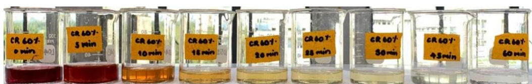
Figure 6 The comparison of effluent from the 1 st -stage decolorization by cation polymer addition treated by ozonation process for 60 minutes
