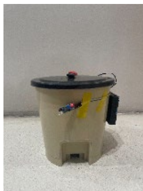
Figure 1. The developed automatic trash bin prototype.
