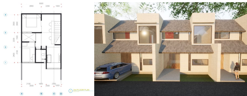
Figure 4. Existing Floor Plan and Appearance of a 2-Story Subsidized House in Bojonegoro Regency Source : Author's Documentation
