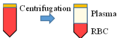
Figure 5. (Centrifugation) The process of separating red blood cells from plasma using a centrifuge.
