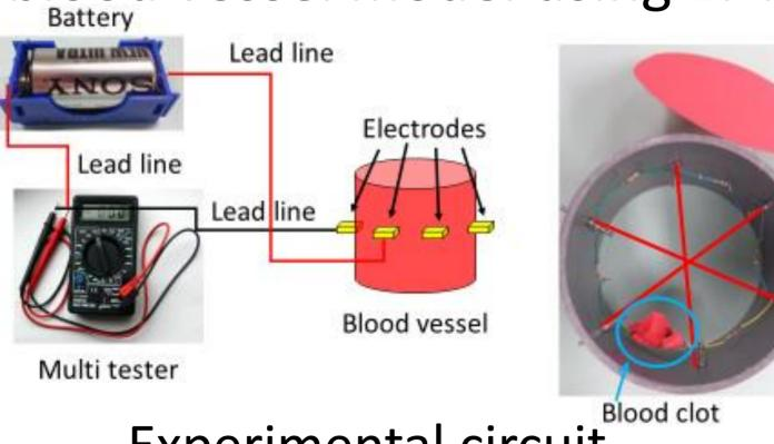
Experimental circuit Make color map based on resistance value High resistance⇒Red
